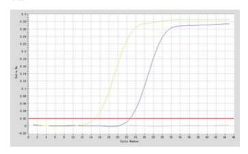
Synthesized standard amplifiction curve (10nM/100pM)
