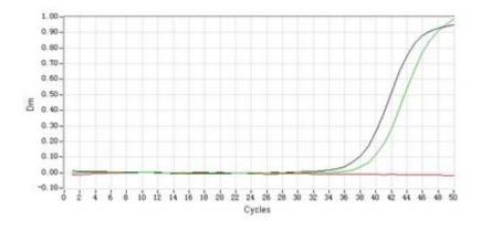
Amplifiction curve in total RNA from cells
