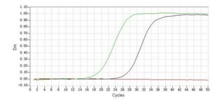
Synthesized standard amplifiction curve (10nM/100pM)
