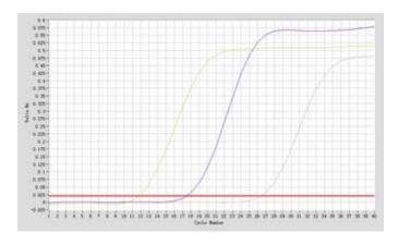
Synthesized standard amplifiction curve (10nM/100pM)
