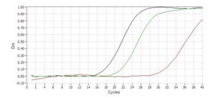
Amplifiction curve in total RNA from cells
