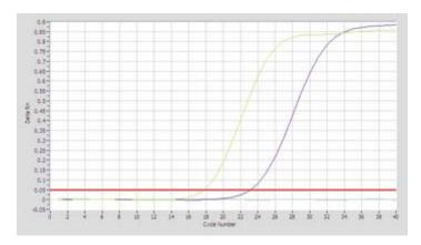
Synthesized standard amplifiction curve (10nM/100pM)
