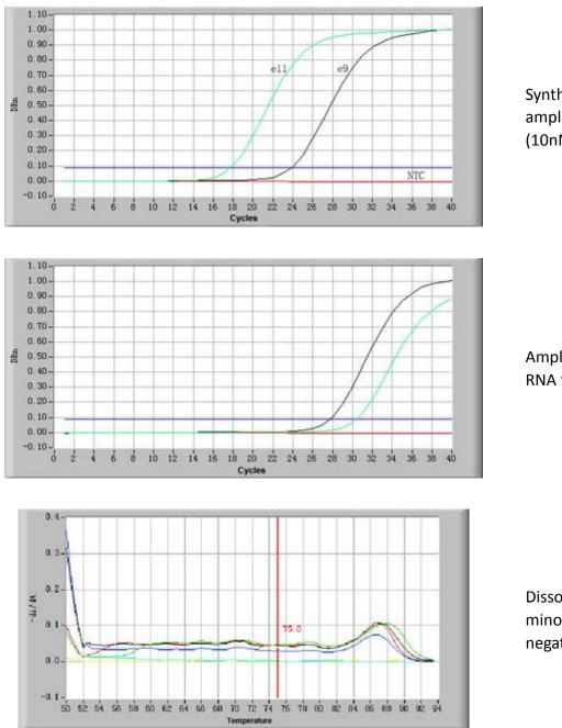
Synthesized standard amplifiction curve (10nM/100pM)
