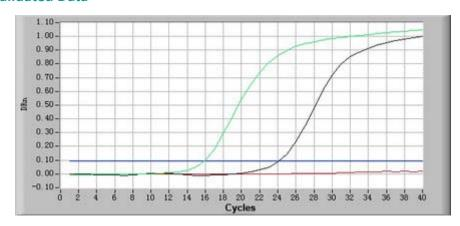
Synthesized standard amplifiction curve (10nM/100pM)
